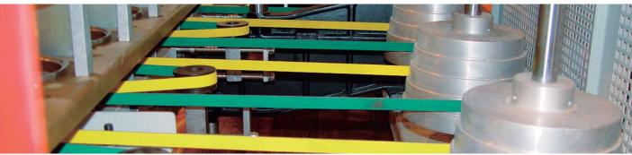
**Keiper CROMA high-performance flat belts** are made of fully synthetic polyamide foils, with a one-sided or two-sided adhesion coating of chrome-split leather.
