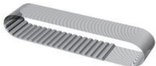
**Keiper PU FLEX timing belts** are extruded endless with helically spooled steel or aramid cords. PU FLEX timing belts exhibit the same high mechanical, chemical and physical properties as our other PU timing belts. Endless, helically spooled timing belts provide a substantially higher transfer of power than endless welded timing belts. Therefore, they can be used for all kinds of power transmission as well as conveying and positioning applications.
