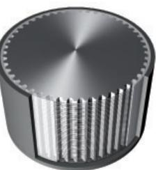
**Polyurethane molded timing belts** (sleeves) are cast in special molds with endless helically spooled steel or aramid tensile cords and thermoplastic polyurethane. In view of the high pitch accuracy along the entire length of the belt, molded timing belts are excellent for power transmission and linear applications, are particularly well suited for smooth running and high speeds.
