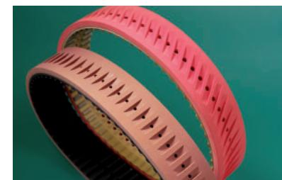
**KEIPER haul-off timing belts**, which are used for conveying foils in bag forming, filling and sealing machines as well as many other conveying tasks, are made with polyurethane or neoprene timing belts in combination with many different kinds of coatings.
