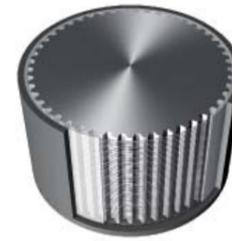
**Polyurethane molded timing belts (sleeves)** are cast in special molds. This ensures very high pitch accuracy along the entire length of the belt, making them particularly suitable for quiet running and high speeds.
