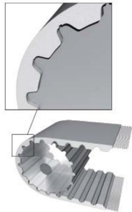
**Polyurethane timing belts**, manufactured in state-of-the-art production processes, are made of abrasion-resistant polyurethane and high-strength steel tension cords, aramid cords or special high flexible HF steel or VA cords.
