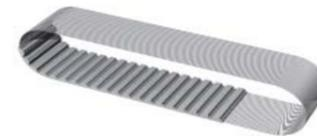
**Polyurethane timing belts "Flex"** are extruded with endless wound cords. For this purpose, the cords are helically spooled. In view of their high power transmission capacity, these timing belts can be used for all types of power transmission as well as many different kinds of synchronous conveying and positioning applications.
