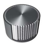
**Polyurethane molded timing belts** (sleeves) are cast in special molds with endless helically spooled steel or aramid tensile cords and thermoplastic polyurethane. In view of the high pitch accuracy along the entire length of the belt, molded timing belts are excellent for power transmission and linear applications, are particularly well suited for smooth running and high speeds.
