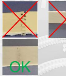
Cables are in contact with the pin; be careful to prevent any cables damages during the installation
