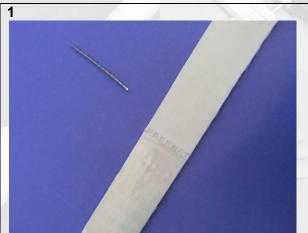
Align the teeth. Teeth must be correctly aligned to avoid any cables damage during pin threading. Misalignment of teeth or the using of a non-chamfered pin can damage the belts cables during the installation
