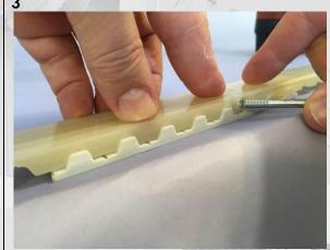
When the pin is completely inserted in the belt, break the pin at the precut area.
