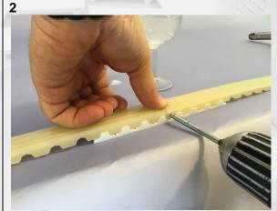
Begin to thread the pin by using an electric screwdriver and water (using as lubricant), to help the threading. For a correct alignment, use the furnished piece of belt, like photo.
