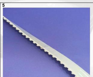
Check that the pin doesn't exceed any edge of the belt.
